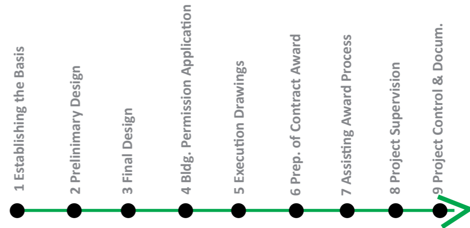
Architect's Traditional Project Understanding according to the German HOAI Service Phases 1-9 (Official Scale of Fees for Services by Architects and Engineers)
