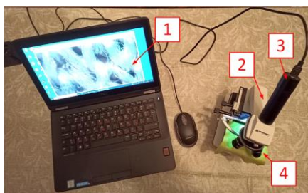
Experimental set-up for obtaining microscopic images - general view. 1-personal computer with software; 2-microscope; 3-video camera; 4-measured sample
